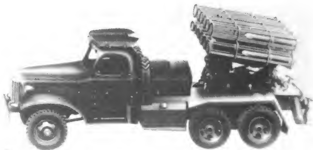
Figure 6-29. Multiple rocket launchers. The 140-mm 16-tube BM-14 (above), towed on a two-wheel carriage, is a standard weapon in airborne divisions. Heavier rockets, such as the 240-mm 12-tube BM-24 (below), are carried on heavy trucks.
